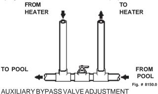
To set bypass: with clean filter, adjustment is made by feeling the inlet and outlet pipes at the heater. Outlet pipes should be slightly warmer than inlet and comfortable to the touch. If pipe is hot, close bypass; if cold open bypass.
